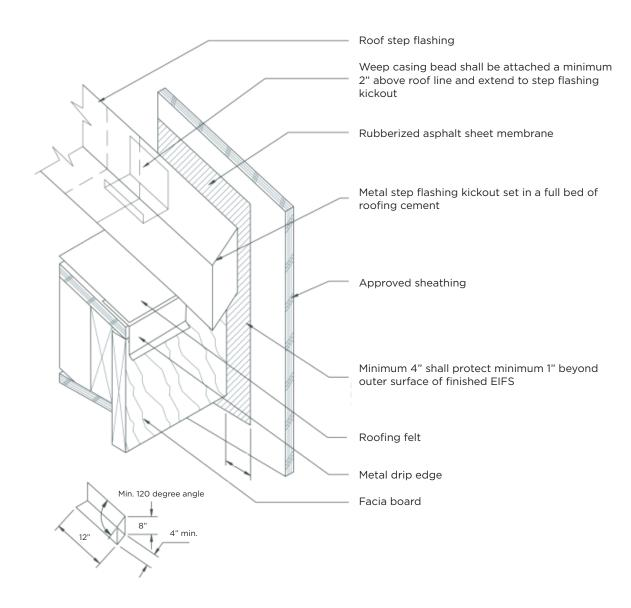
NOTE 1: The "kick-out" diverter flashing must be installed prior to installing the water managed EIFS system. NOTE 2: Do not install the outer system until the water managed EIFS system has been completed.
